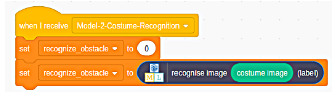
Fig. 6. Example Scratch code in our self-driving car tool to employ Model 2 for image detection.
